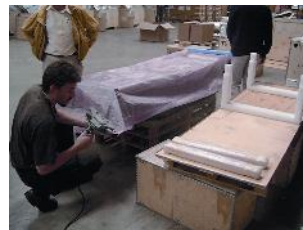
CPS solution : ESD foil, foam dunnages Box : NEFAB ExPak H + 2 1/2 perimeters and lightweight pallet
