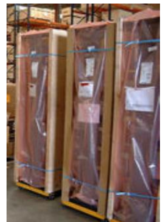
CPS solution : ESD foil, foam dunnages Box : NEFAB ExPak H + 2 1/2 perimeters and lightweight pallet
