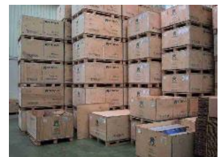
Stacking capacity increased from three to eight boxes with the new Nefab solution
