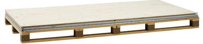
Nefab ExPak XL is made of high-quality birch or pine plywood, 8-12 millimetres thick depending on the application. When collapsed for storage, it takes up very little space. This packaging can be used with most types of pallets, making it very flexible. Nefab has tested the concept's resistance to compression, vibration, impacts and falls in its own packaging lab.
