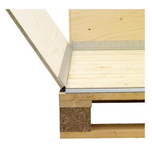
The side panels are mounted using a profile that is pressed into their lower edge. The panels can be mounted horizontally onto the base profile or be angled inwards up to 60°, reducing the need for a lot of space when packaging goods.
