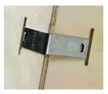
The packaging is held together with clamps, which are mounted without tools in the pre-cut grooves. The clamps are made of flexible sprung steel, so they don't pop off when the packaging is bumped or jolted. All that is needed for dismantling is a regular screwdriver; the clamp is designed to drop right into your hand rather than flying off and potentially hurting someone.
