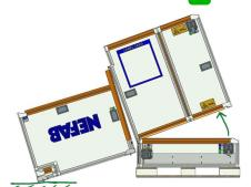
Open lower front latches. Let top hood pivot back onto floor.
