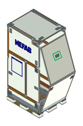
Lower until front door is fully folded and rests on the ground.
