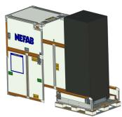
Fold the rear flap underneath the hood and lower onto floor.
