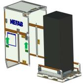
Using four lower handles, carefully lift hood
