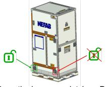
Open the lower rear latches. Do not open the lower front latches!
