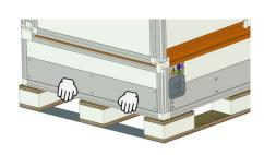
Swing hatch upwards and hold in place
