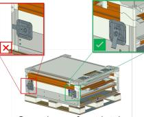
Open lower front latch. Do NOT open rear latch.
