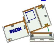
Rotate panels downwards into base profiles
