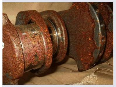
For products transported under tough conditions with significant humididty and temperature changes, humidity control and corrosion protection are needed.
