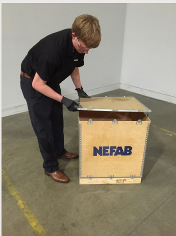
Step 3: Place the lid over the top with the tabs in the lid slots. Bend the tabs with a screwdriver. The top tabs should be bent down towards the floor. The bottom tabs should be bent upwards toward the sky.
