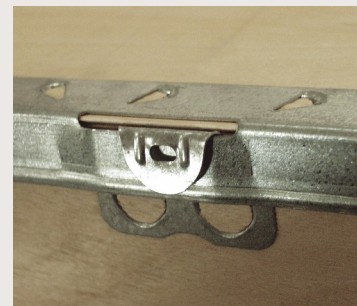
To open and close the box, place the end of a screwdriver in the hole in the tab and bend it 180 degrees.
