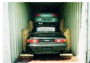
Dunnage bags can even be used with stacked transport sets.
