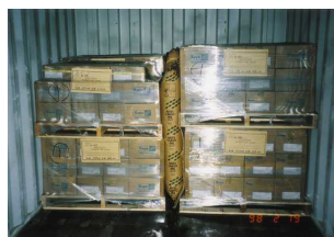
Dunnage bags prevent damages by blocking goods inside a load carrier.
