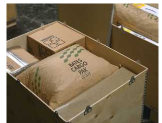
Dunnage bags can be even used inside a ExPak/RePak.
