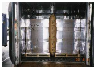
Dunnage bags adapt to different shapes of pallet loads.
